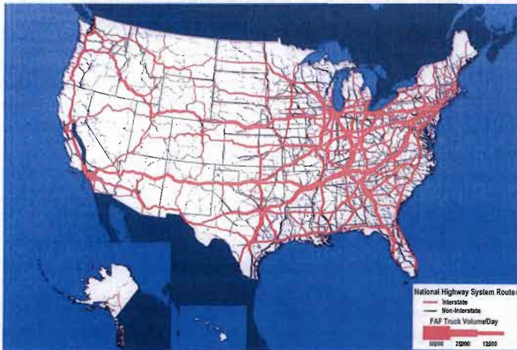
Figure 2.2: Average Daily Long-Haul Freight Truck Traffic on the National Highway System: 2007
